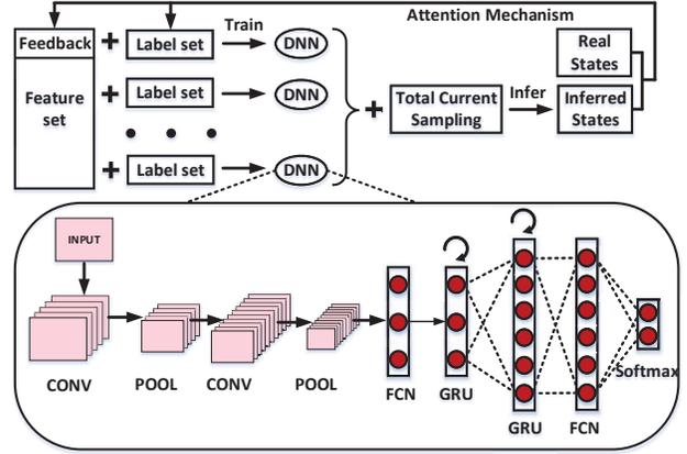
Figure 7. The training procedure and the structure of DNN
