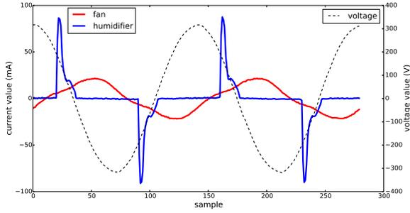
Figure 4. Current waveforms of fan and humidifier
