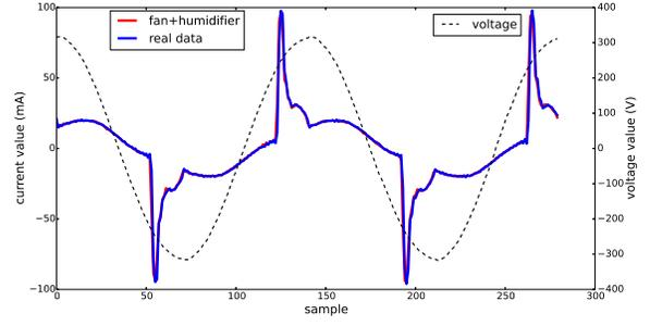
Figure 5. Actual and constructed current waveforms of fan add humidifier
