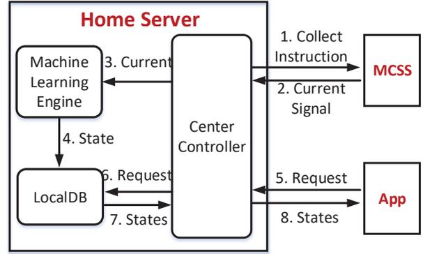
Figure 2. The data flow diagram of normal working
